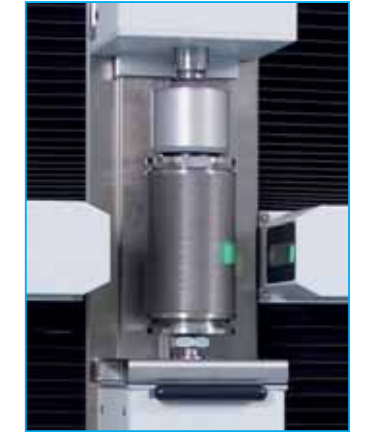
CONTOUR AUTOMATIC 310, cylinder liner application
