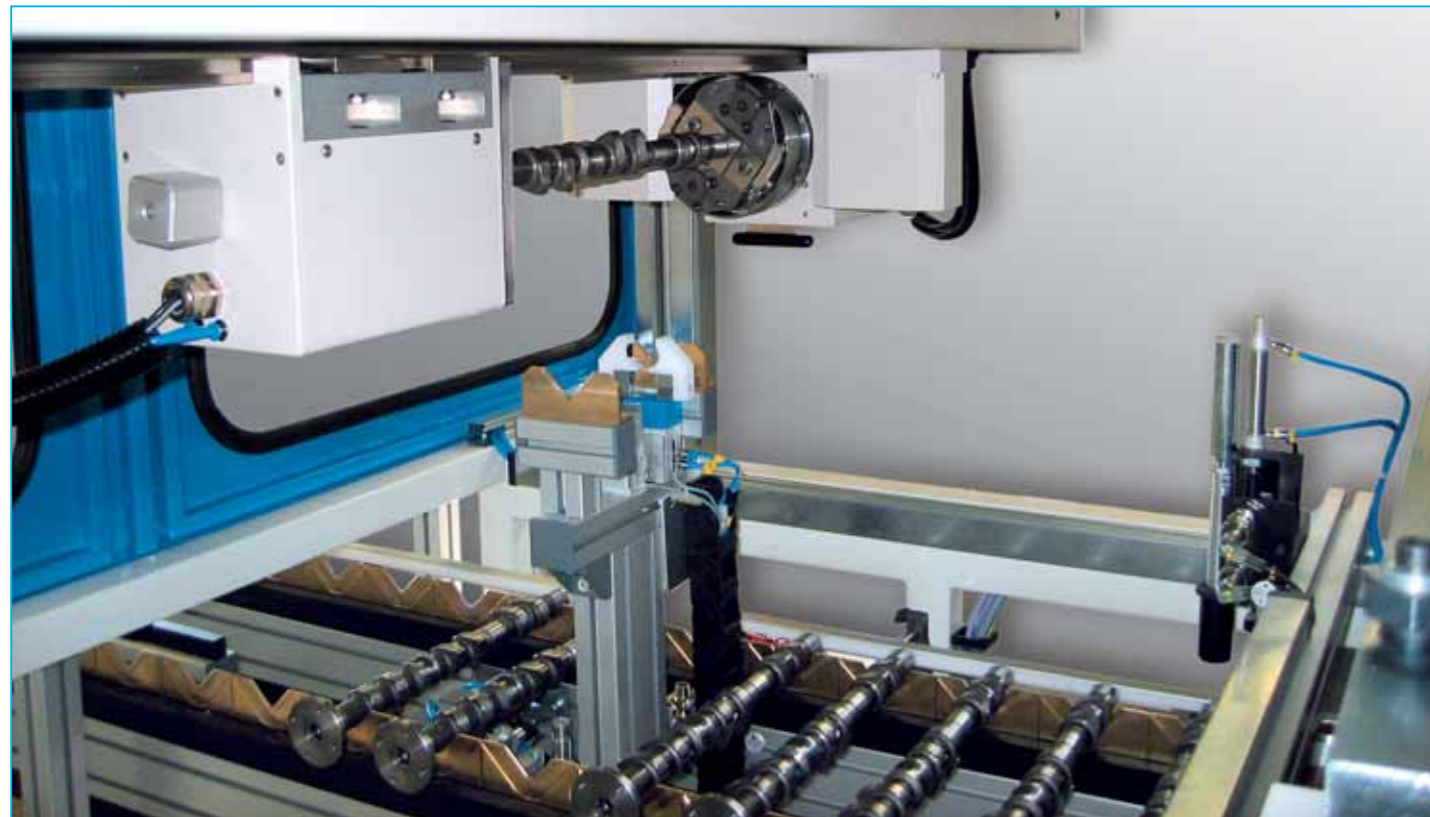
CONTOUR AUTOMATIC 810H, cam shaft application
