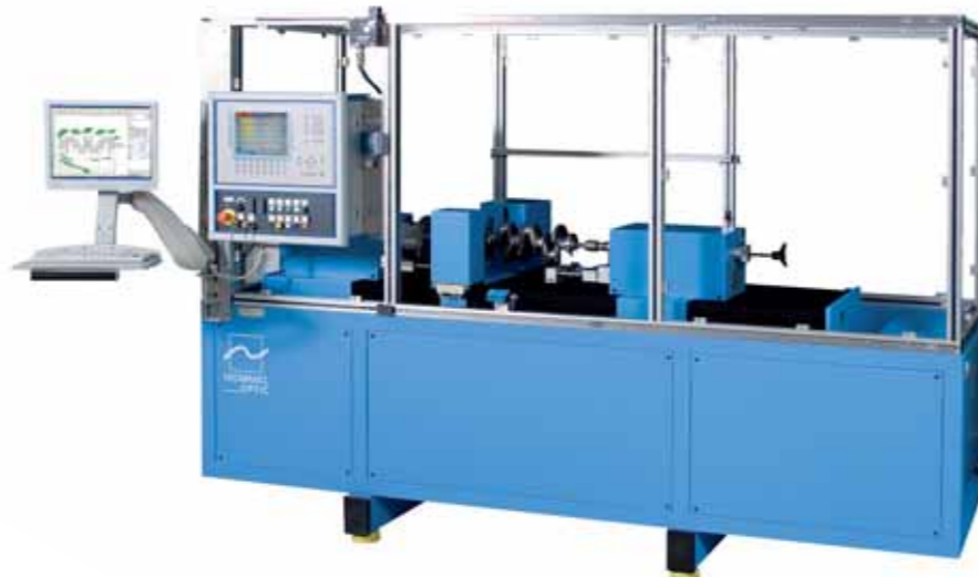
AMV 923H, crank shaft application, for concatenated post-process work sequence measurement
