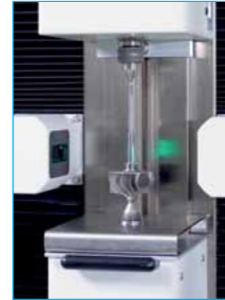
CONTOUR AUTOMATIC 305, turbocharger application
