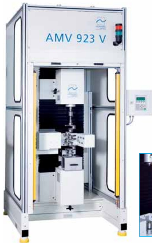
AMV 923V, crank shaft application with robot loading
